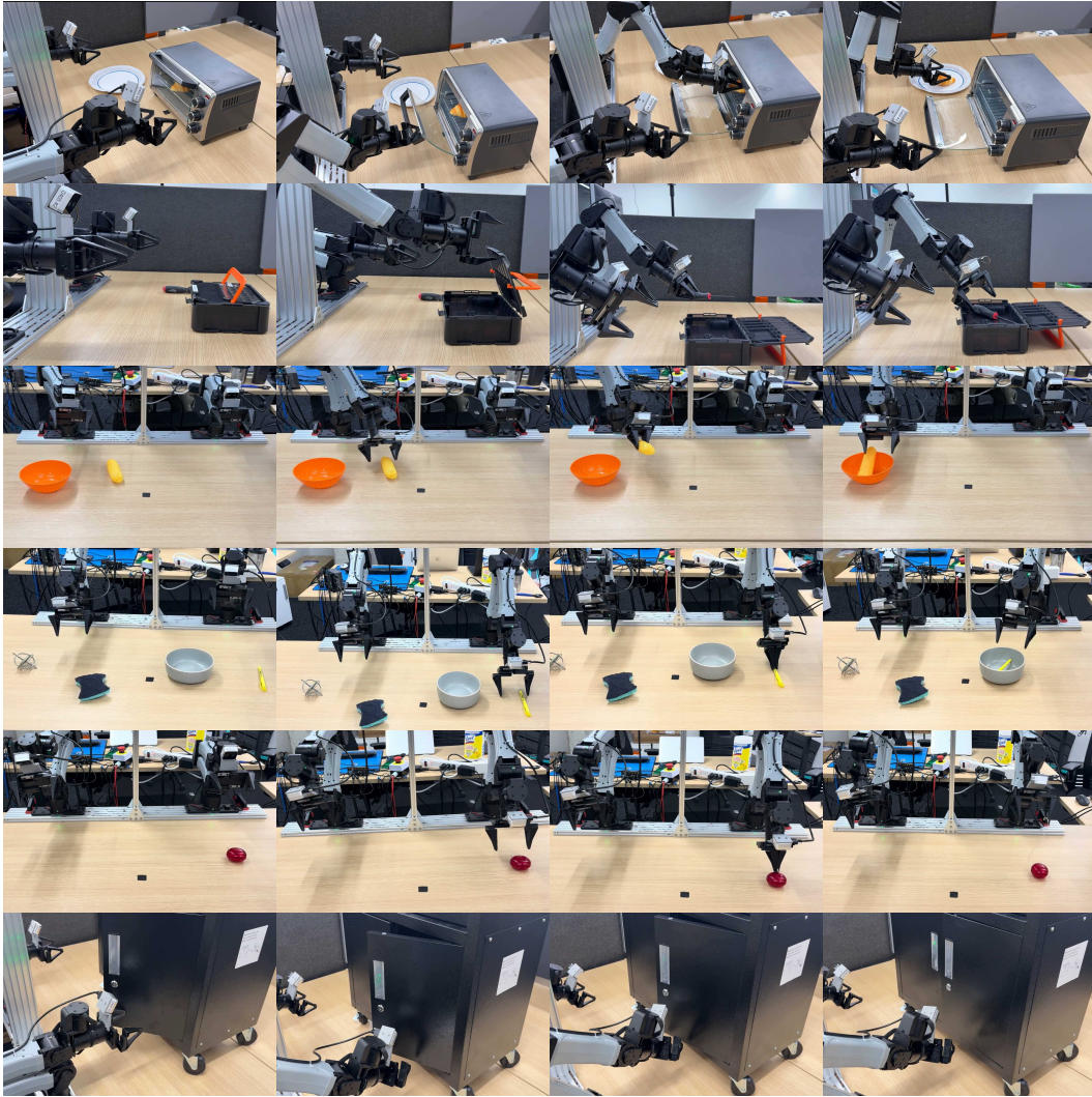
Figure 6: Rollout videos. Each row shows intermediate progression of successful FloMo rollouts of different tasks (3 in-distribution and 3 OOD). (a) The top row is opening the oven and placing the croissant on a plate. (b) The second row is opening the toolbox and placing the screwdriver inside. (c) The third row is placing the corn in the bowl. (d) The fourth row is putting the highlighter in the bowl (OOD task). (e) The fifth row is pulling the string on a toy (OOD task). (f) The last row is closing the cabinet (OOD task).
